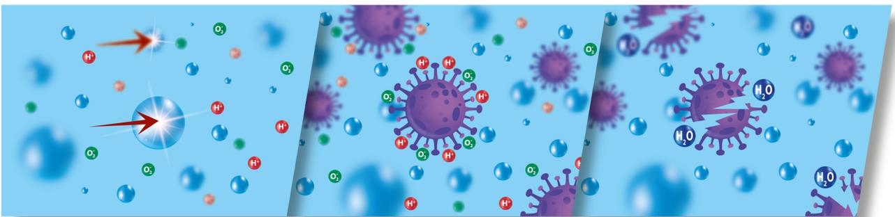
Ionisation is a process carried out by applying a large quantity of energy (in the form of electric potential or radiation) to the atoms to generate molecules that are positively charged (positive ions) or negatively charged (negative ions). The ionised gas is called "plasma".
